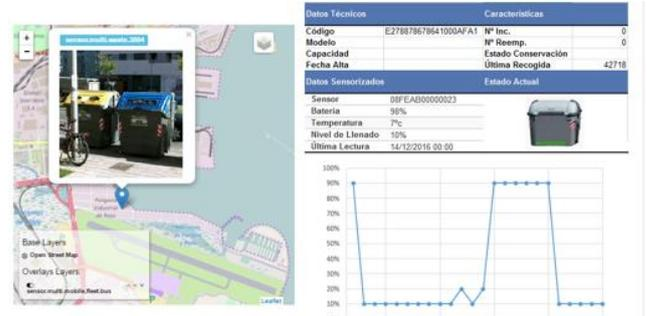
The system analyzes data, based on needs, in order to increase or decrease the frequency at which they come by depending on the capacity and condition of the containers.
